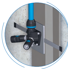
FASTENED TO IPN/HEA BEAM WITH PLATES
