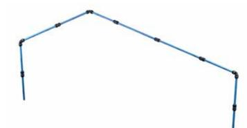
Pressure: 8 bar | Max. pressure drop 5% (0.4 bar) | Max. speed: 10 m/s
