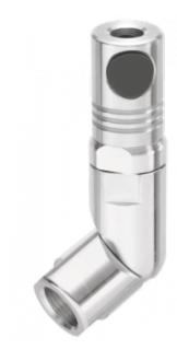
**BSPP** female thread **Technology Operating pressure** Flow rate at 6 bar 833 l/min (?P = 0,6 bar) G 3/8 Safety (avoid hose whip) 0 to 16 bar **ID Passage** Construction Highlight **Temperature** -15°C to +70°C Body: Stainless steel 6 mm Anti-static
