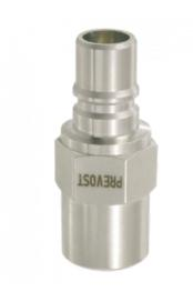
ID Passage (mm) **BSPP** female thread Max operating **Temperature** G 1/4 +15°C to +200°C pressure 16 bar Construction **Applications** Ø 6 - 9 - 12 mm : Brass, Ø Cooling circuits, cleaning, 16 mm: Stainless steel and rinsing, food processing chromium industry
