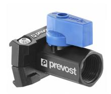
For pipe ID (mm) **BSPP** female thread **Technology Operating pressure** G 1/2 **PPS Grip Concept** 0 to 16 bar Vacuum capability **Temperature** Construction Highlight -0.98 bar (vacuum 98%) -20°C to +80°C Pipe and fittings: alu. Scalable system Meets standards PED REACH
