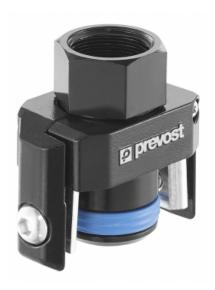
For pipe ID (mm) **BSPP** female thread **Technology Operating pressure** 25 G 1/2 PPS Grip Concept 0 to 16 bar Vacuum capability Construction Highlight **Temperature** -20°C to +80°C -0.98 bar (vacuum 98%) Pipe and fittings: alu. Scalable system Meets standards PED REACH
