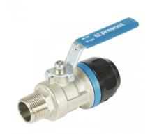
For pipe OD (mm) Technology **BSPT** male thread **Operating pressure** R 1/2 **PPS Grip Concept** 0 to 16 bar Vacuum capability Construction Highlight **Temperature** -0.98 bar (vacuum 98%) Pipe and fittings: alu. -20°C to +80°C Scalable system Meets standards PED REACH
