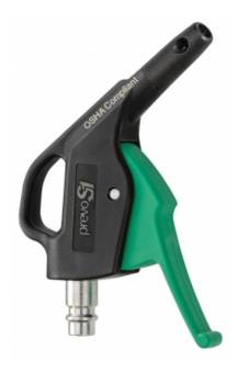
Blowing force (at 6 bar Dynamic pressure (at 10 Air consumption (at 6 Sound level (at 6 bar mm at 6 bar (bar)) bar (Nm3/h)) (dBA)) 260 13 87 Max operating pressure Construction Highlight Temperature -15°C to +70°C 12 bar Polyamide composite body Compact Connection Built-in adaptor
